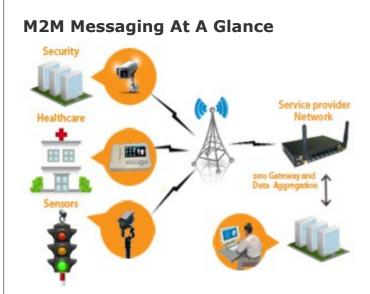
Machine-to-Machine (M2M) technology has been around for quite some time. M2M Messaging is one of the M2M services that allows automated machines to communicate and send messages to each other or to other devices.
